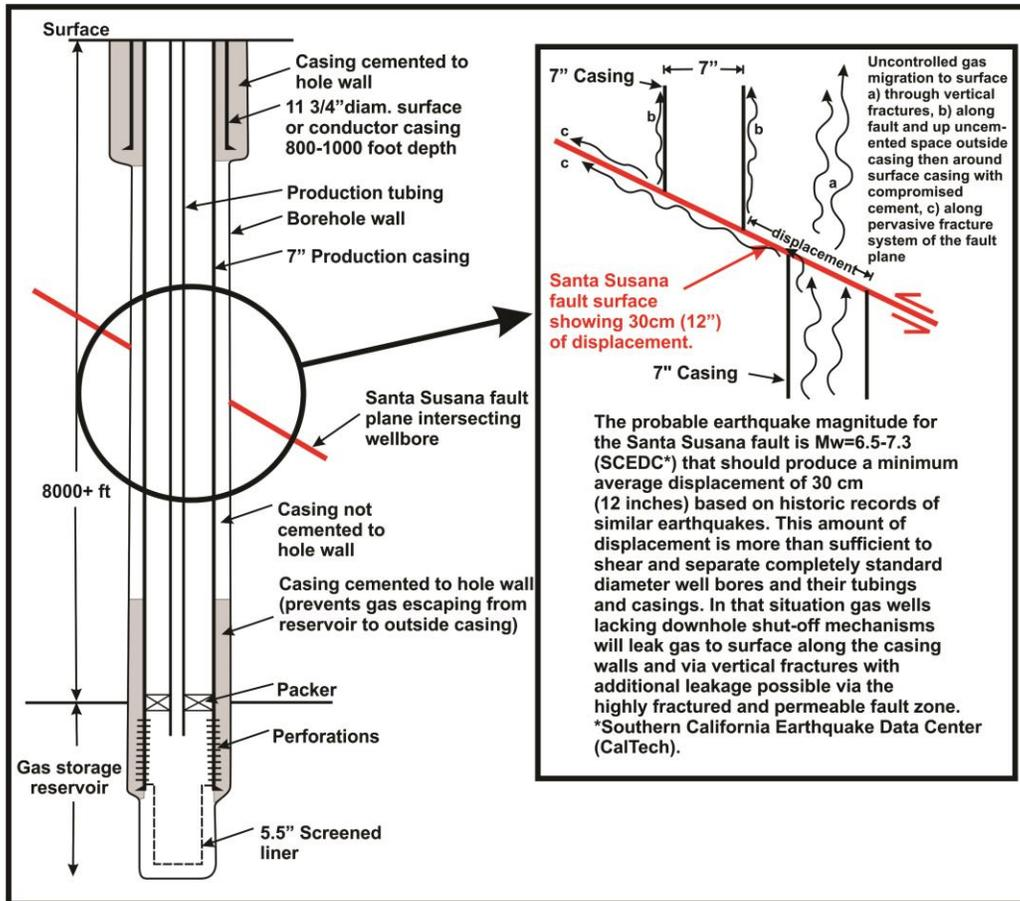
Figure 1. Well schematic showing a gas storage well at the Aliso Canyon Gas Storage Field on the left. Diagram on the right shows a postulated earthquake sourced fault displacement along the Santa Susana fault offsetting the well and postulated methane migration pathways to the atmosphere from the damaged well.
