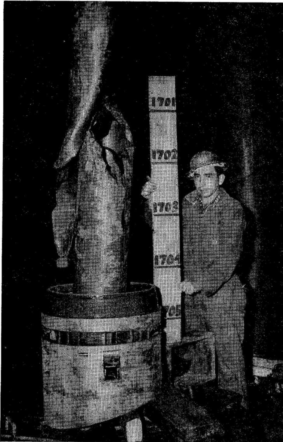
PLATE IV. Union Pacific Railroad Company well No. "Union Pacific" 403, Sec. 3, T. 5 S., R. 13 W., S. B. B. & M. Deformation of 10 $\frac{3}{4}$ " casing at 1701' ("K<sub>1</sub>"). Recovered by washover tool. Date: February 23, 1950.
